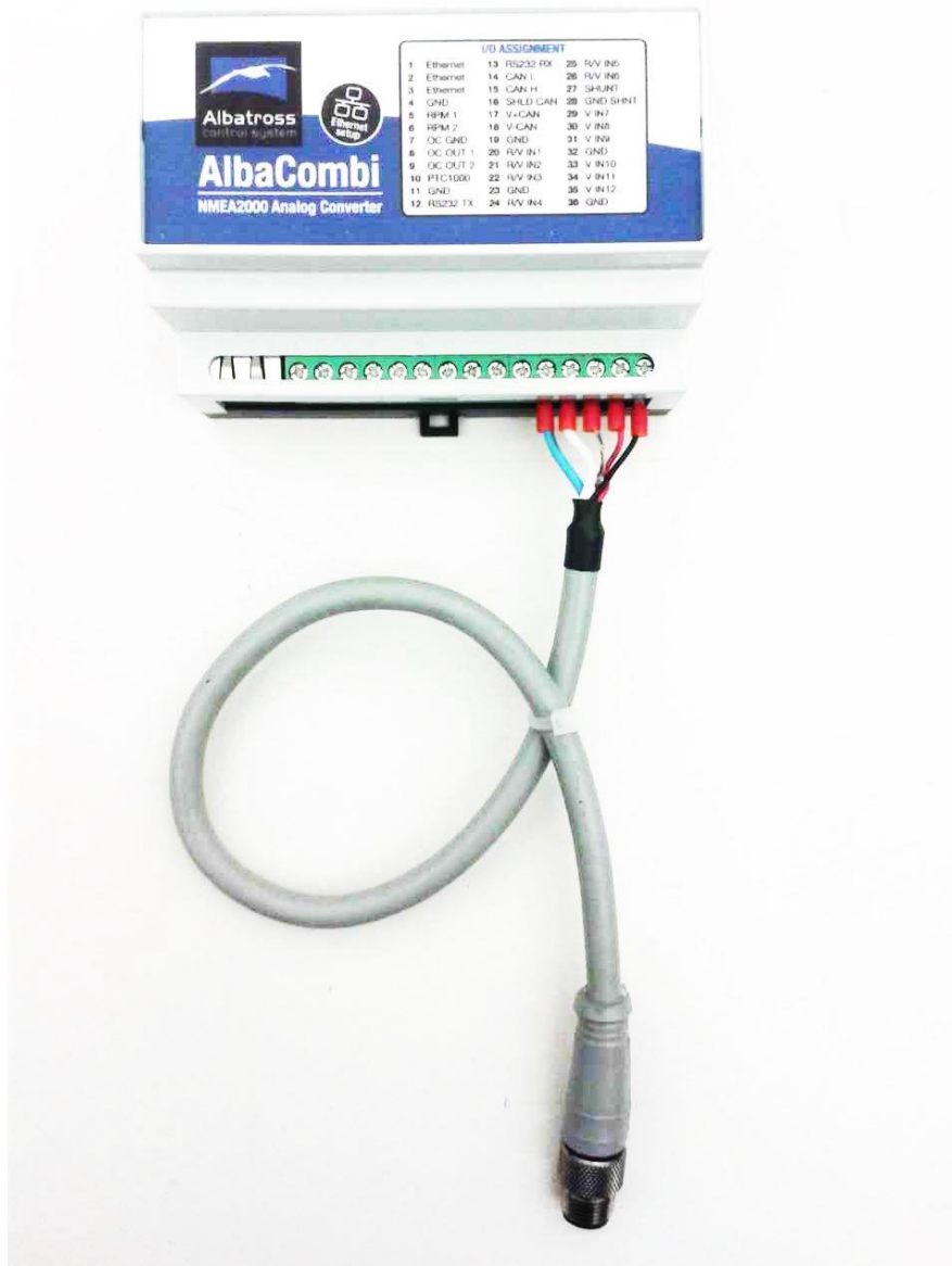
Normal connection with a NMEA2000 Spur Cable
